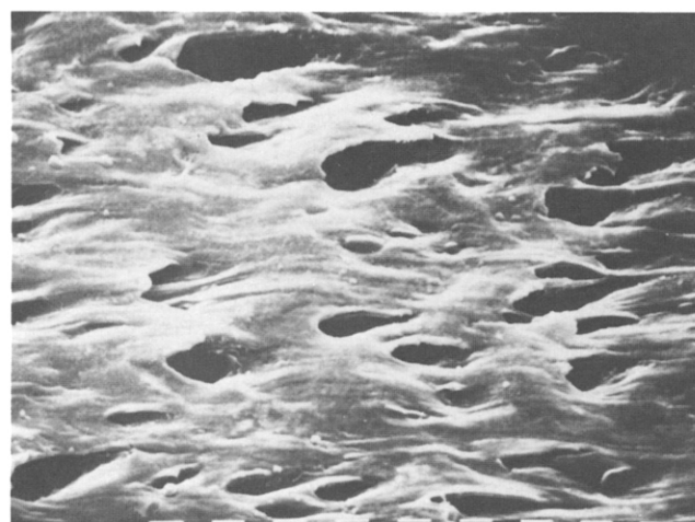
Figure 7 Scanning electron micrograph (3600 \times ) of a smoothed HDPE/EP-12 sample surface etched for 3 min with boiling n-heptane vapour
