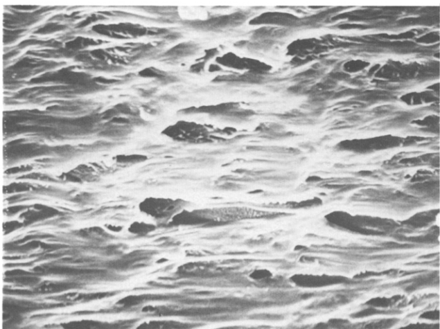
Figure 6 Scanning electron micrograph (3600 \times ) of a smoothed HDPE/EP-45 sample surface etched for 1.5 min with boiling n-heptane vapour
